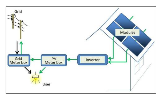
Figure 126: main components of a PV system
