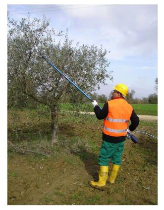
Figure 87: operator using a pneumatic shear mounted on a rod and wearing personal protective equipment
