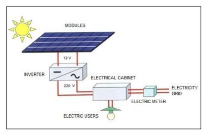
Figure 130: grid-connected system
