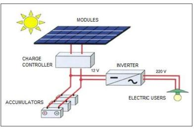
Figure 129: stand-un Alone or Off-Grid system
