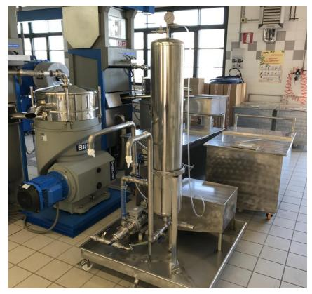
Figure 116: vertical separator and column filter
