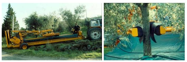
Figure 109: trunk shaker with trailed interceptor frame
